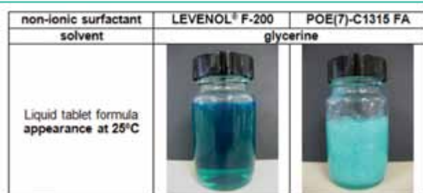
Figure 4. Formula appearance at 25°C of liquid tablet formulations with glycerine. Left: with LEVENOL® F-200 (clear liquid), right: with POE-fatty alcohol (turbid paste). Formula composition (65% active): 27.3% non-ionic surfactant, 19.5% MEA-Cocoate, 7.3% SLES, 10.9% MEA-LAS, 20% glycerine, q.s. other ingredients.
